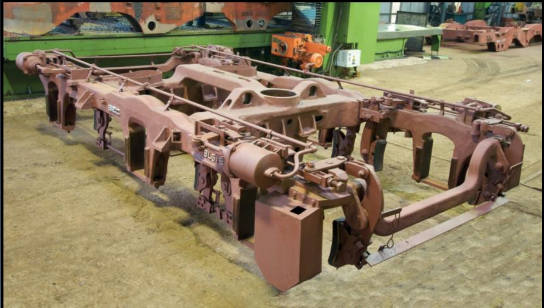
Cast Steel Locomotive Bogie Frame Assembly ( 6½ ton)
